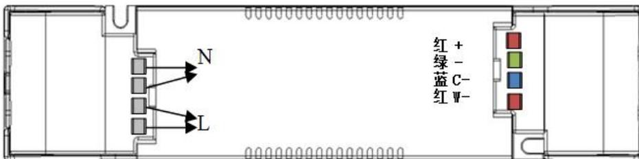
In the power line L, the TRIAC Dimmer can be connected in series to achieve dimming.
